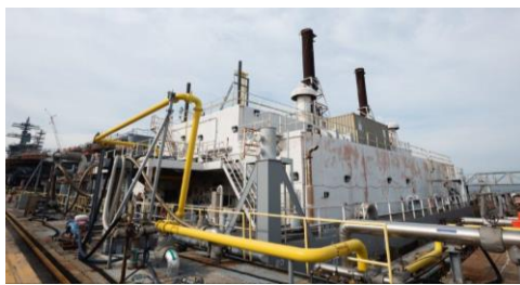
Newport News Shipbuilding converted a steam barge from liquid fuel to natural gas, significantly reducing emissions
