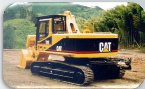
Tunneling Tethered Electric Excavator
