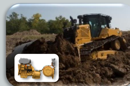
D6 XE Elevated Sprocket Electric Drive
