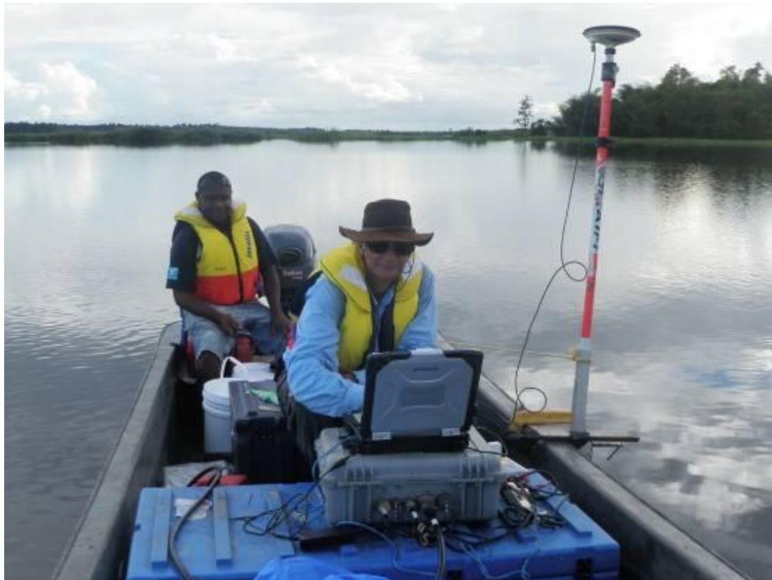
Figure 0-6 Typical hydroacoustic set up
