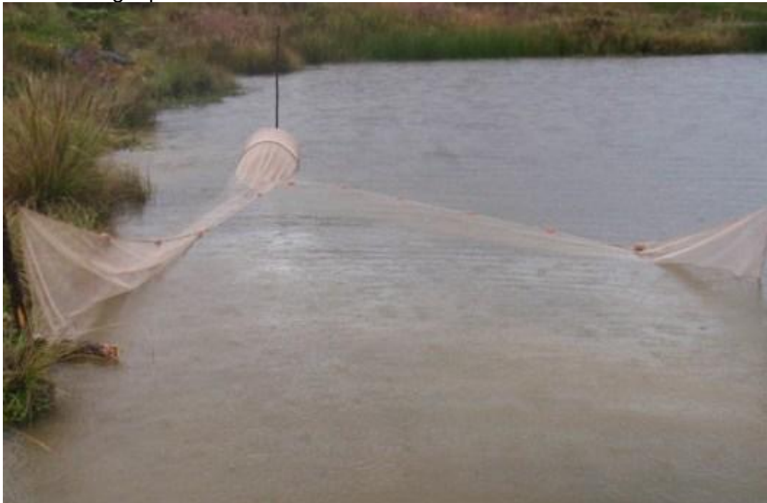
Figure 0-5 Typical set up of fyke net used for sampling prawns and fish during 2010
